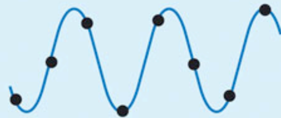
Sampling the analogue signal
