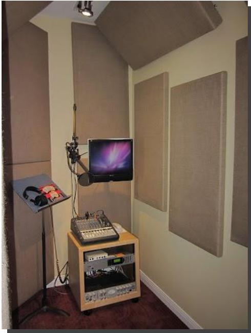
The larger the room, the lower its resonant frequency, just like a larger bottle has a lower pitch, and a bass violin needs to be larger than a violin to create a powerful bass note. A small space, such as a linen closet, small walk-in closet, or an isolation booth from WhisperRoom, will resonate very heavily in the low to mid-range frequencies of your voice. This is partly what creates that “boxy sound”, but there’s more to the
